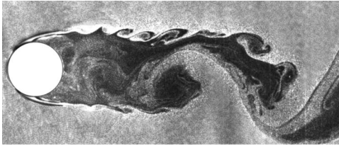
FIG. 4. Instantaneous thickness field in the wake behind a cylinder. Maximum thickness variation 50% of mean thickness, with darker areas corresponding to thinner film. d=2590 \mu\text{m} , u_\infty=170 \text{ cm/s} , h=12.7 \mu\text{m} , \nu=3.7\times 10^{-2} \text{ cm}^2/\text{s} , and \text{Re}=1200 . The width of the field is 16 mm.
